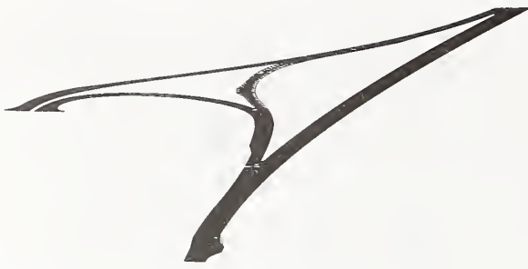
Figure 3: The 3-D surface model created for the tests. The model was designed by Terra Street CAD application and used directly to control the blade of grader.
